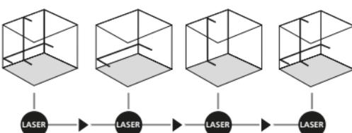
The transport restraint must be released for horizontal and vertical levelling. The LED (2) shows a permanent green light. The laser lines flash and the LED (2) lights red as soon as the device is outside the automatic levelling range of 5°. Position the device such that it is within the levelling range. The LED (2) switches back to green and the laser lines stop flashing (steady light).
